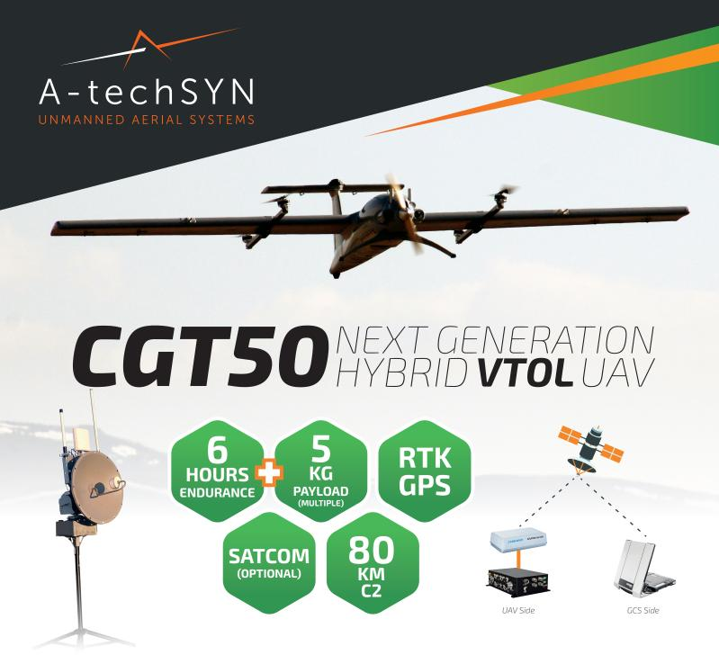
The **CGT50-SLT** is a 4.71 m wingspan T-Tail UAV. It uses electric powered motors for takeoff and landing and does not require a runway or catapult. It is a composite airframe with 5 kg payload capacity, powered by a petrol engine. The low fuel consumption enables a safe endurance of 6 hours. The **CGT50-SLT** can takeoff from a table and land on a 5x5 m surface with high accuracy.
